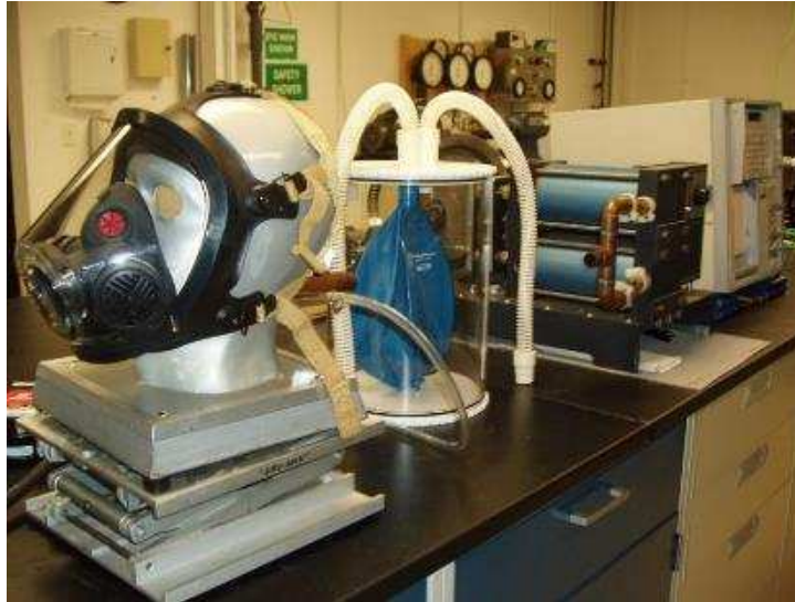
Supplied-air Peak pressures with 40 LPM breathing machine
