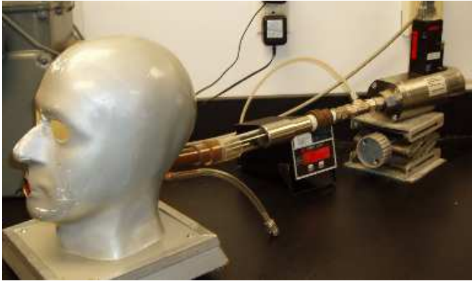
Air-purifying Air-flow Resistance at constant flow ( \pm 85 LPM)
